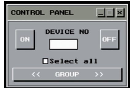
Fig. 2: Control panel screen for switching the device either 'on' or 'off'
