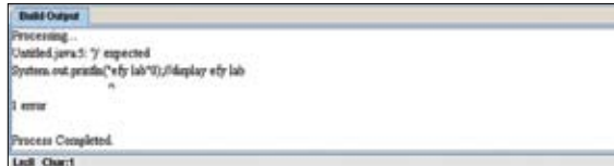
Fig. 8: Typical message display in build output window
